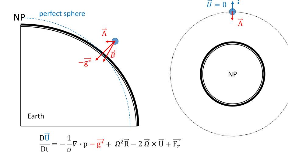
Consider a 'motionless' atmosphere to an observer at Earth's surface (i.e. the observer is rotating around the Earth's axis of rotation)
