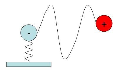
Oscillations in the electric and magnetic fields move, "radiate", through space.
