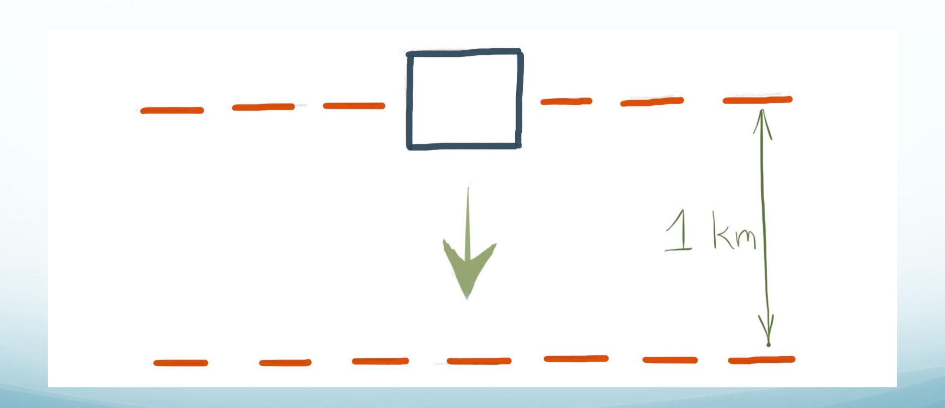
The environmental lapse rate is 5° C per km. A dry air parcel given an initial push downward from a height of 1 km. It will tend to keep moving downward.
