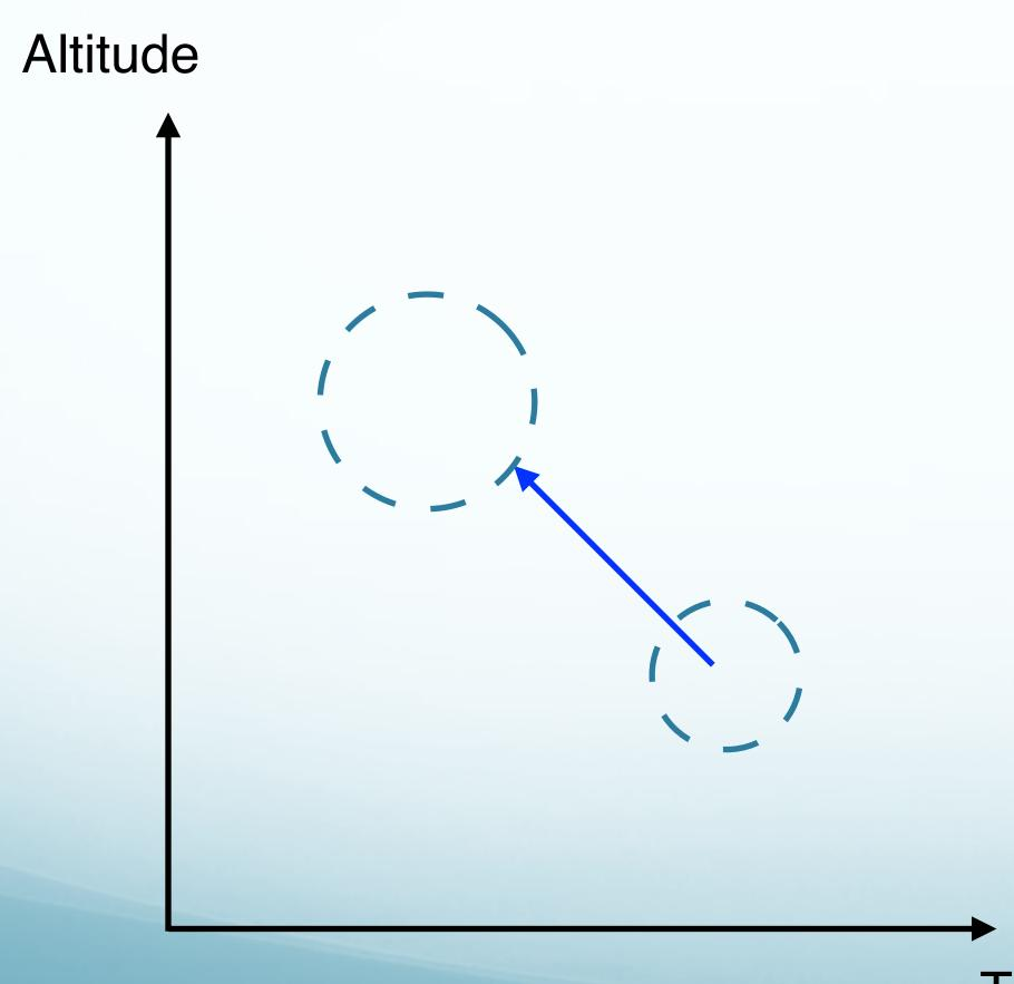
Dry adiabatic lapse rate: the rate at which temperature drops in an air parcel as it is adiabatically raised up (always 10 °C/km)
