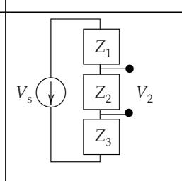
$$T(s) = \frac{V_2(s)}{V_s(s)} = \frac{Z_2}{Z_1 + Z_2 + Z_3}$$
