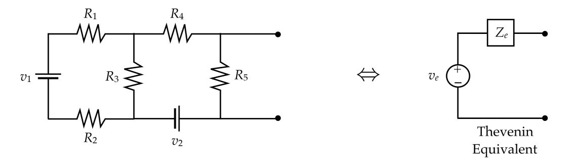
$v_{\rho}$  = voltage that appears across the open-circuited terminals of the network
