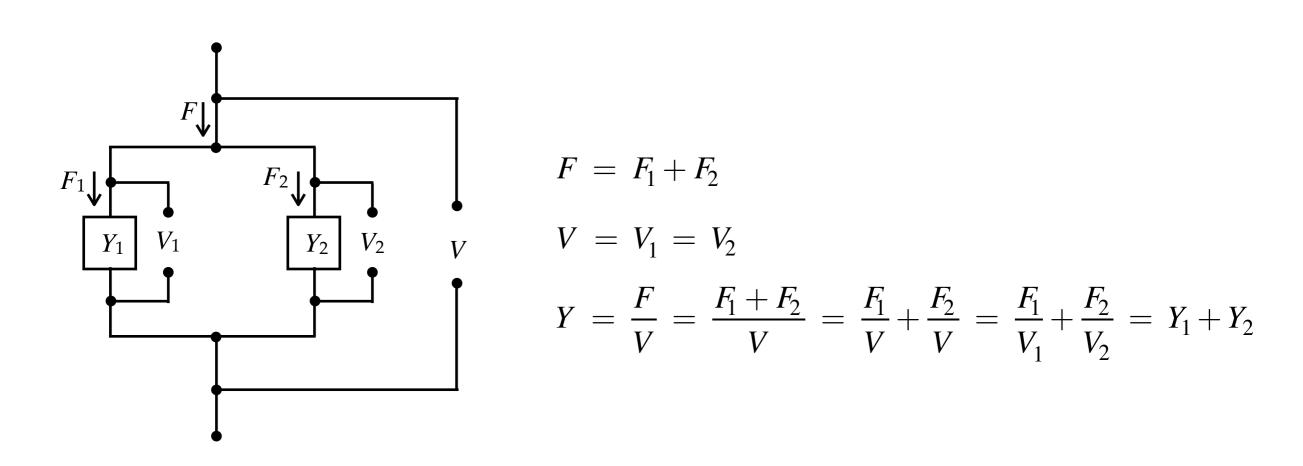
Series and parallel combinations of impedances and admittances can be combined. In the following *V* and *F* represent the across and through variables respectively of any physical domain.
