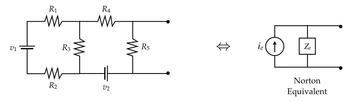
$i_e$  = current that would flow through the short-circuited terminals of the network
