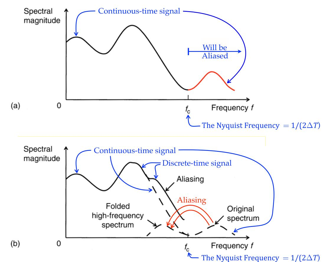
Figure 3.14 Aliasing distortion of a frequency spectrum. (a) Original spectrum. (b) Distorted spectrum due to aliasing.
