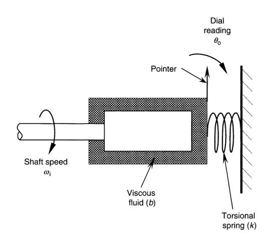
Assumption: The power in via the rotating shaft goes into (1) friction losses between the rotating cylinder and the fluid, and (2) the potential energy stored in the torsional spring:
