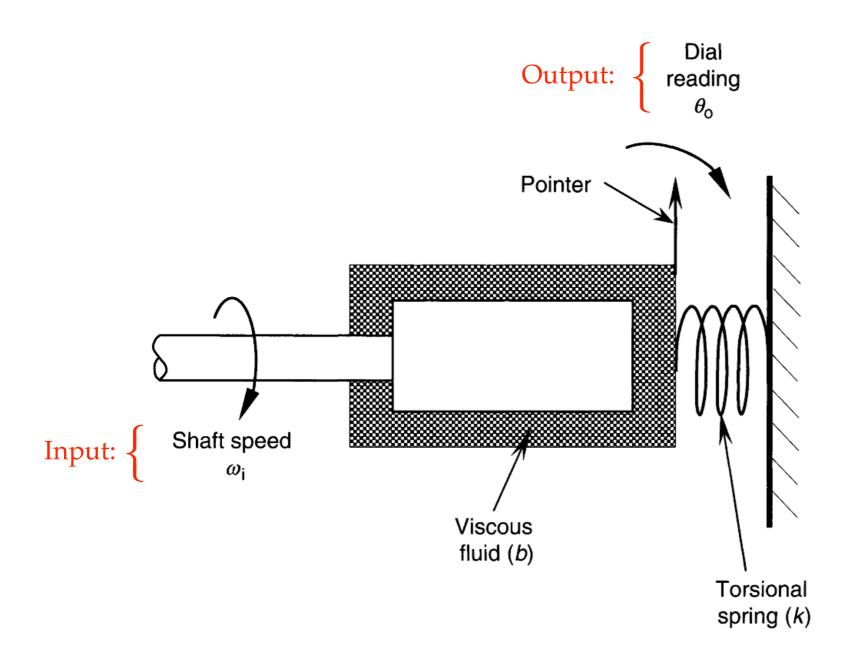
Figure 3.13 A mechanical tachometer.
