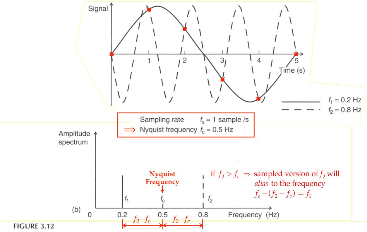
A simple illustration of aliasing: (a) two harmonic signals with identical sampled data. (b) frequency spectra of the two harmonic signals.
