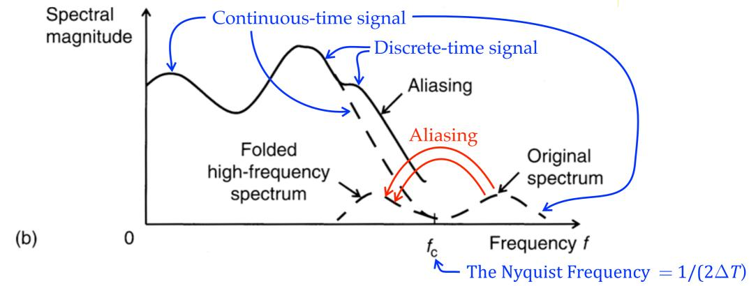
Figure 3.14 Aliasing distortion of a frequency spectrum. (a) Original spectrum. (b) Distorted spectrum due to aliasing.
