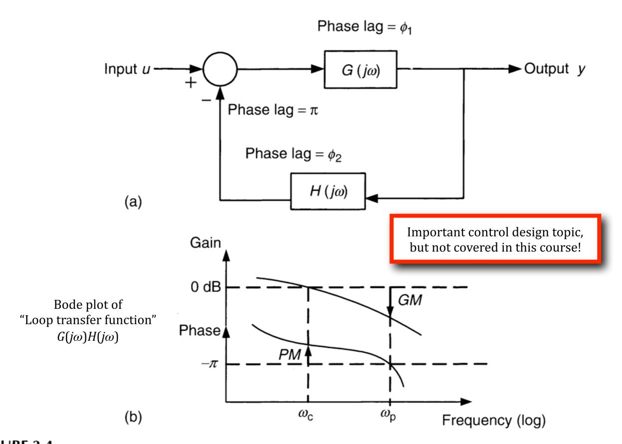
**FIGURE 3.4** Illustration of gain and phase margins. (a) A feedback system. (b) Bode diagram.
