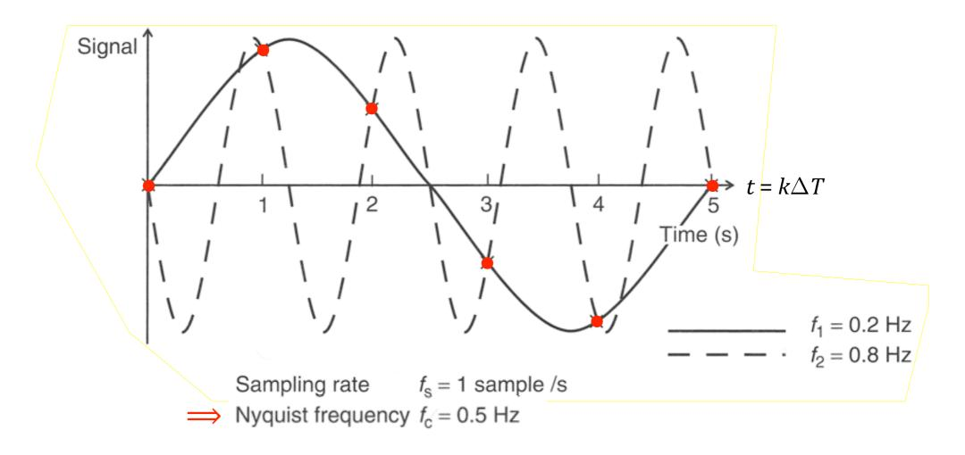
The signal  $\cos(2\pi ft)$  is sampled at  $\Delta T = 1$  sample/s to produce the sampled signal  $\cos(2\pi fk)$  (that is,  $t = k\Delta T$ , for k = ..., -2, -1, 0, 1, 2, ...). What frequencies f are aliased to  $\cos(2\pi f_1 k)$  for  $f_1 = 0.2$  Hz?
