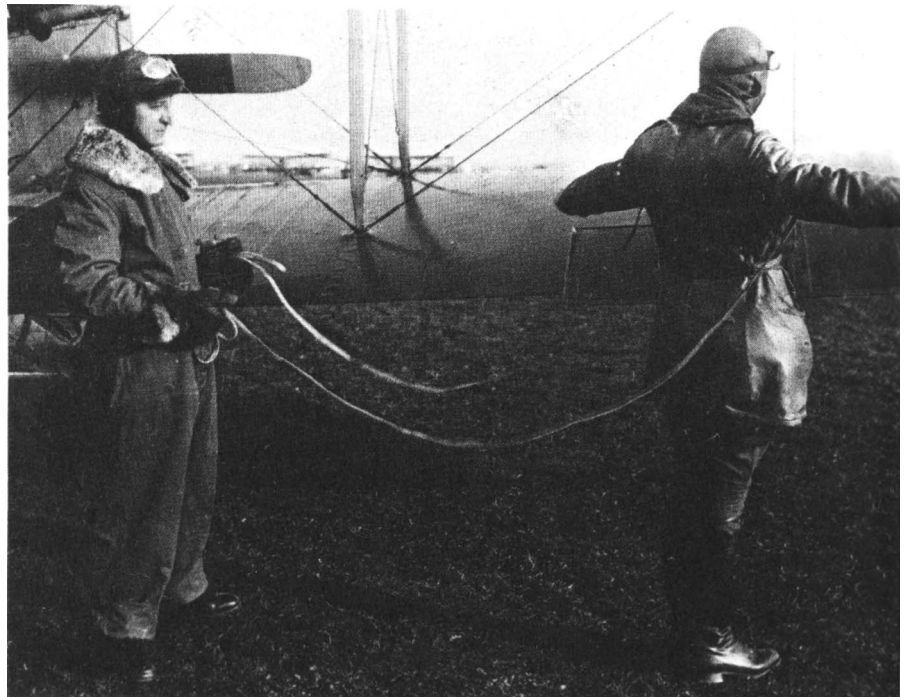
Figure 1. An observer and pilot demonstrating an early, physical-based, steering system for communicating directions. Source: US Air Force Historical Studies Office.
