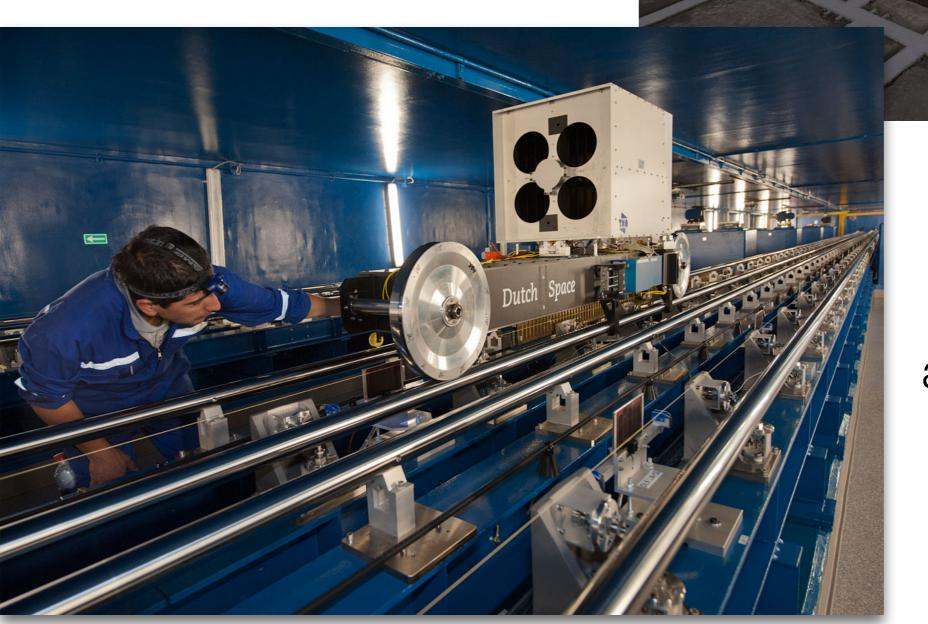
Must be kept in alignment to less than a micron
