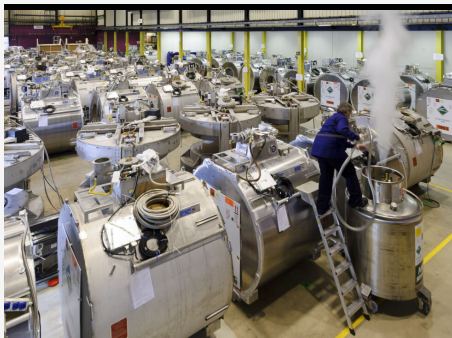
MRI magnets under construction at the Philips Healthcare production facility in 2010. [credit: Jock Fistick/Bloomberg via Getty Images ]
