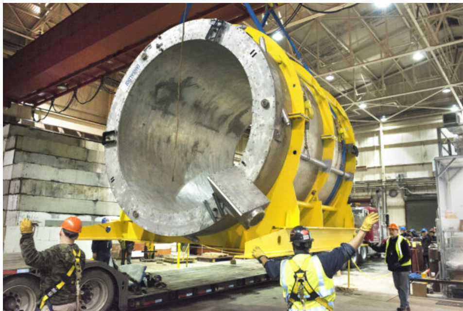
Enlarge / A superconducting magnet used for a particle detector.
