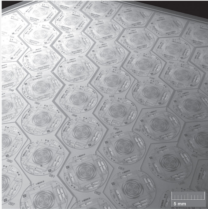
Superconducting sensor array for the South Pole Telescope Cosmic Microwave Background telescope. [credit: IOP Science ]
