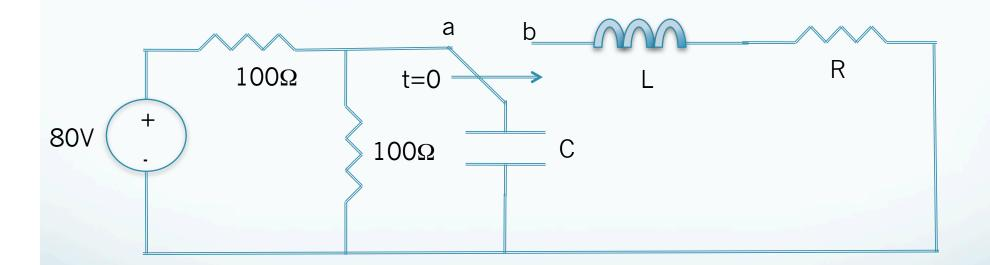
This circuit is an RLC circuit which goes into its Natural Response at t > 0Unlike the previous RLC circuit, however, this is a series RLC circuit (rather than a parallel RLC circuit)
