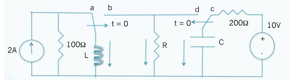
After the switch is in position b for a long time, and After the switch in position d for a long time. The capacitor becomes an open circuit. The inductor becomes a short circuit.
