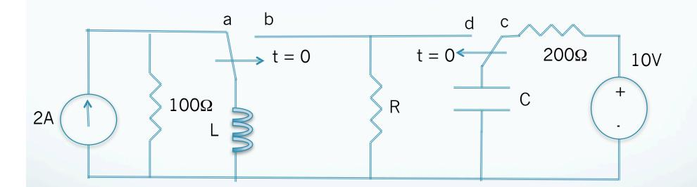
This circuit is an RLC circuit which goes into its Natural Response at t > 0
