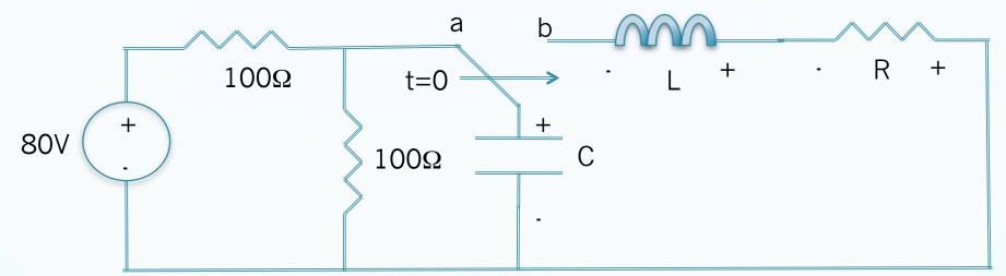
After the switch is in position b for a long time, and The capacitor becomes an open circuit. The inductor becomes a short circuit.
