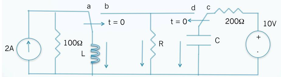
Once we know the form of the solution by analyzing the roots of the characteristic equation, we can solve for the unknown coefficients in the differential equation via the initial conditions of the circuit.
