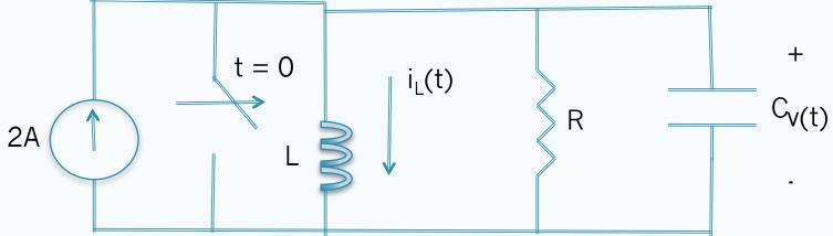
At t>0, power is applied to the circuit. This circuit can be analyzed similarly to the natural response of the parallel RLC circuit. We can use an approach that makes the analysis very similar to that for the natural response.
